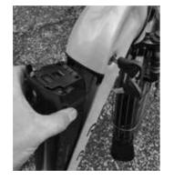
Step 3 Grip the top of the battery and lift out of the frame.
