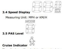
The display will calculate the actual travelling speed based on the wheel diameter and signal data (number of magnetic steel is needed for Hall motors)
