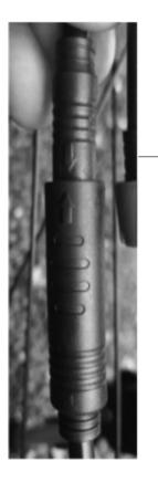
Motor QR plug: Press here to release then pull apart.
