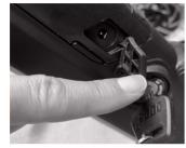
**To charge the battery** - The battery can be charged either on or off the bike using the charge point as shown located next to the battery lock.
